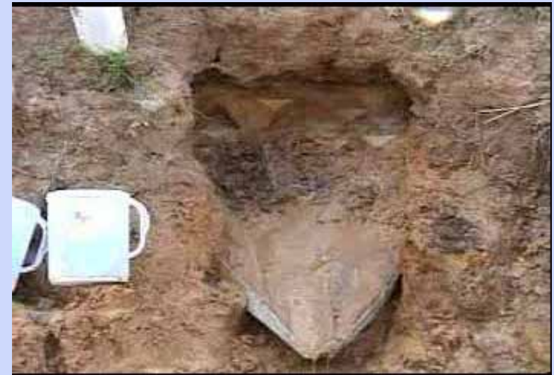
Seepage Flow/Sediment Measurements with Lateral Flow Collection Pans
