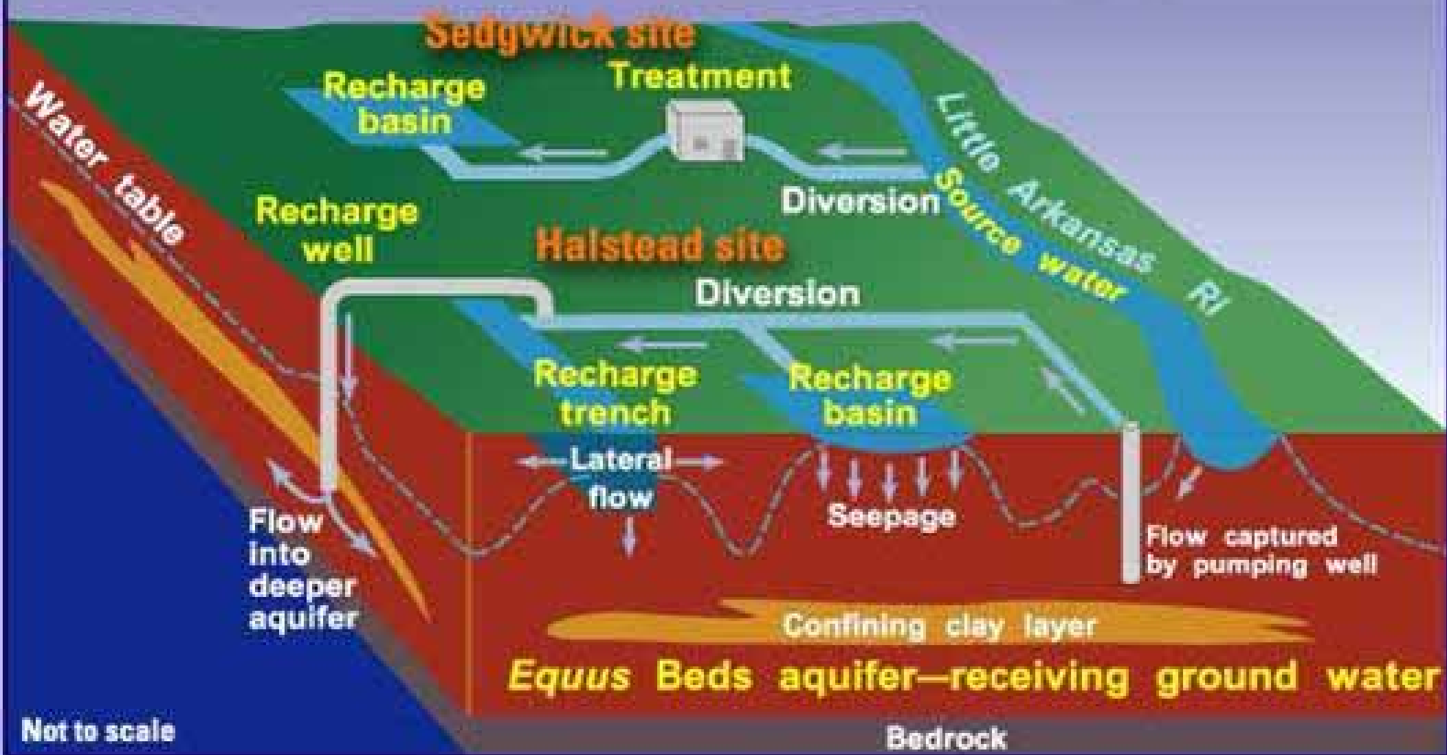
Schematic of the artificial recharge process. (USGS, 2001)
