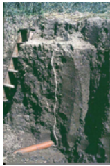
Macropore Connected to Drain (Picture courtesy of V. Nuutinen and K. Butt)
