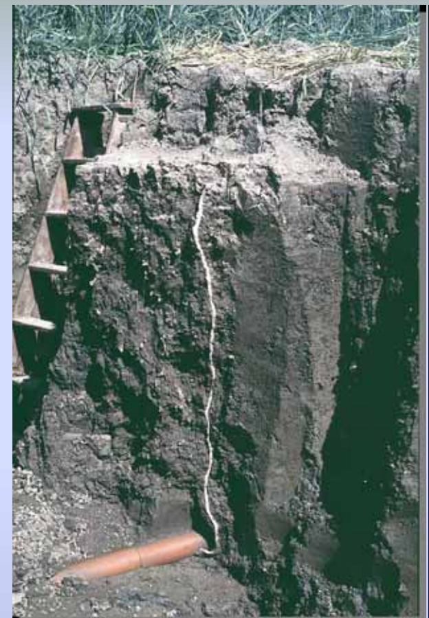
Macropore Connected to Drain (Picture courtesy of V. Nuutinen and K. Butt)
